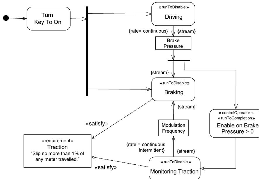
Vertical and horizontal bars in Figure 3 are forks showing initiation of concurrent flows of function invocations. For example, after the key is turned on, driving and braking functions start concurrently, because the control flow coming out of TURN KEY TO ON is split into two concurrent control flows, to DRIVING and BRAKING. The SysML keyword «runToDisable» on a function invocation indicates that once the function starts, it runs until it is turned off (turning the key to off is not shown).
