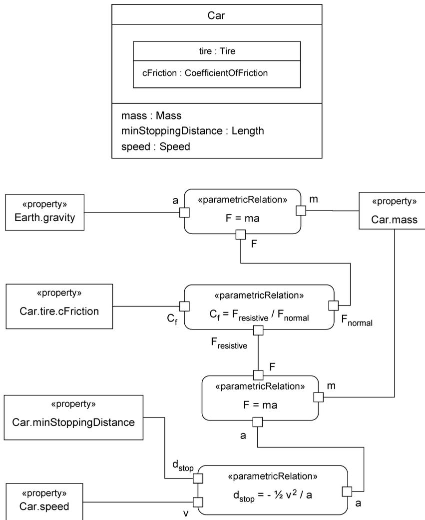
For compactness, parametrics can be notated as equations, and still be stored to the SysML repository. Tools can use the repository to generate the equations from diagrams such as Figure 5, or vice versa. The SysML repository does not dictate or suggest
