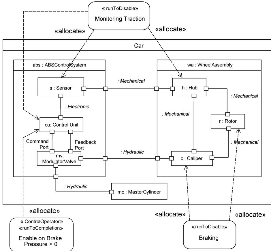
As usual in model-driven approaches, other notations for allocation can be supported, for example to show functions inside the part rectangles, or in a tabular format, and so on. UML also supports a notation that groups the steps in an activity, called *partitions*, which can be also used for allocation (Bock, 2004a).
