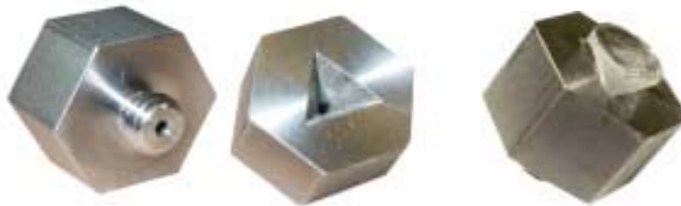
Figure 2. Titanium holder before and after the small retroreflector was mounted
