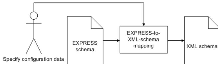
Figure 1. Converting an EXPRESS schema into an XML schema using Part 28
