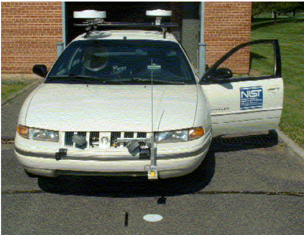
Figure 1 Note the downward looking photo sensor, the retroreflector on the ground and the vertical rod to guide the driver.
