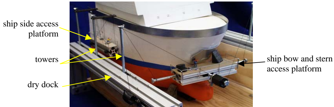
Figure 1 – NIST Flying Carpet 1/120 th scale concept model showing the ship bow/stern access configuration (right) and the ship side-access configuration (left).
