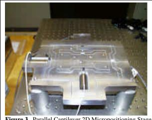
Figure 3. Parallel Cantilever 2D Micropositioning Stage
