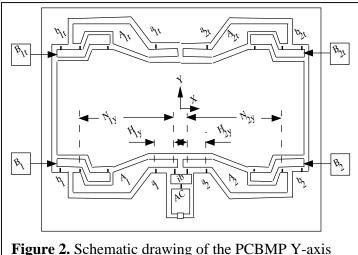
motion mechanism with a folding cantilever.
