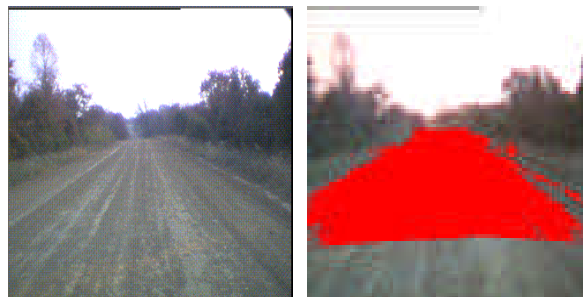
Figure 5. Color image and projected area of both lidar and color label as road
