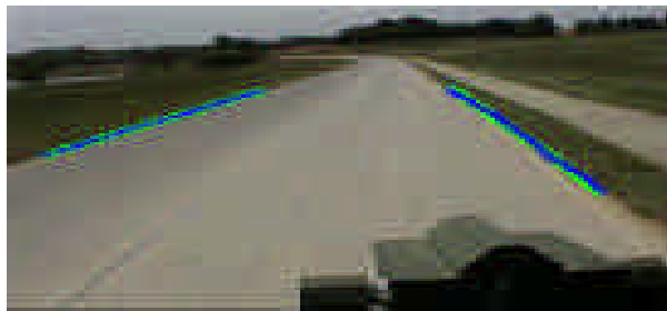
Figure 4. Initial road boundary. Blue points are road edges, green points show the model fitted to the boundary
