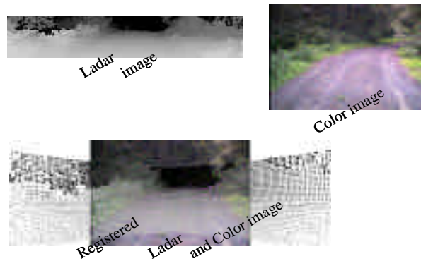
Figure 7. The mapping between Ladar data and color data
