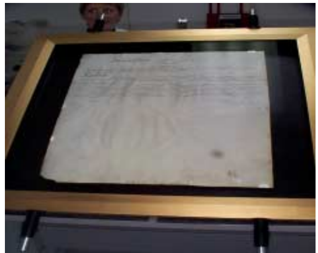
Figure 1. The first prototype encasement, shown here with the transmittal page for the Declaration of Independence. Sized for the Bill of Rights, the encasement can accommodate the smaller document, albeit with asymmetric margins.
