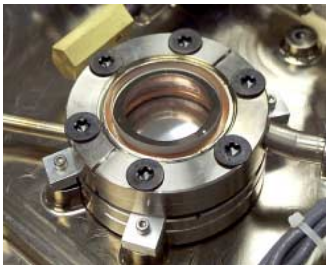
Figure 3. In case of an unexpected pressure differential The rupture disk is designed to fail before the main glass.
