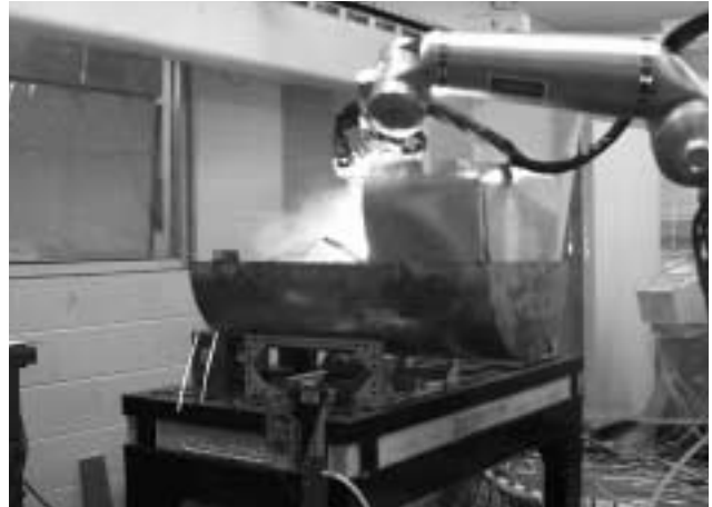
Figure 1. The remote welding testbed.
