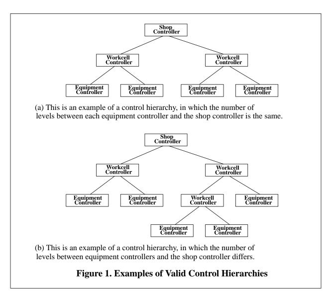
There must be production plans for every level of control, except possibly for the equipment level. For equipment controllers which use machine-specific programs, production plans are not generated; the higher level production plans specify the scheduled execution times of these programs.
