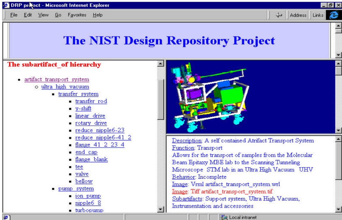
Fig. 7. A sample user interface. The graphical screen depicts one VRML view of the overall system. The lower screen describes the system, its basic function and its subartifacts. The system hierarchy is listed on the left.
