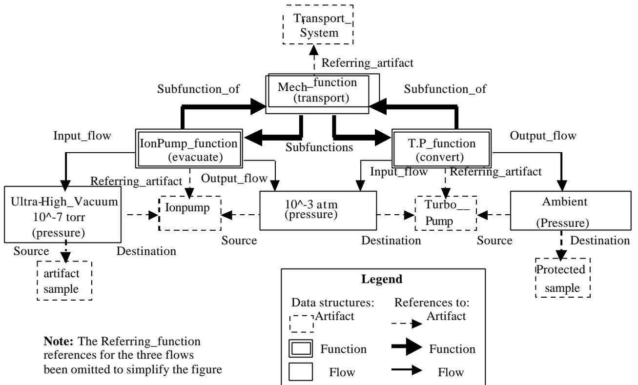
Fig. 6. Graphical representation of ultra-high vacuum pump function.
