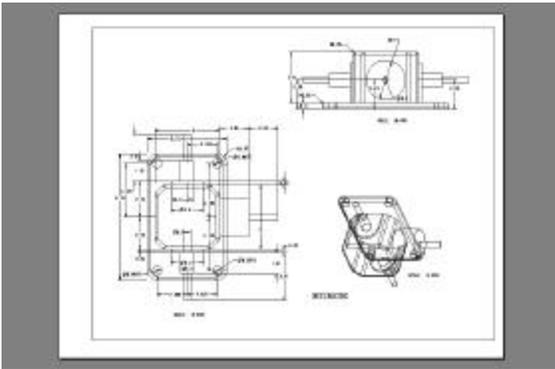
**Fig. 2.** Typical CAD drawing of a mitre gear box. This component was one of four deployed for the jacking system.
