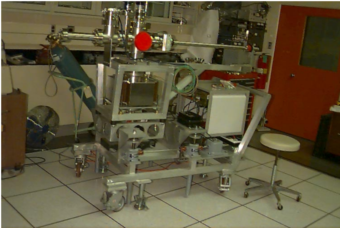
Figure 2. Photograph of the constructed cart and UHV systems in the STM Laboratory.
