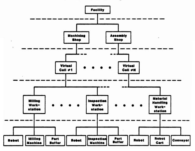
Figure 2. Expanded AMRF Control Hierarchy.
