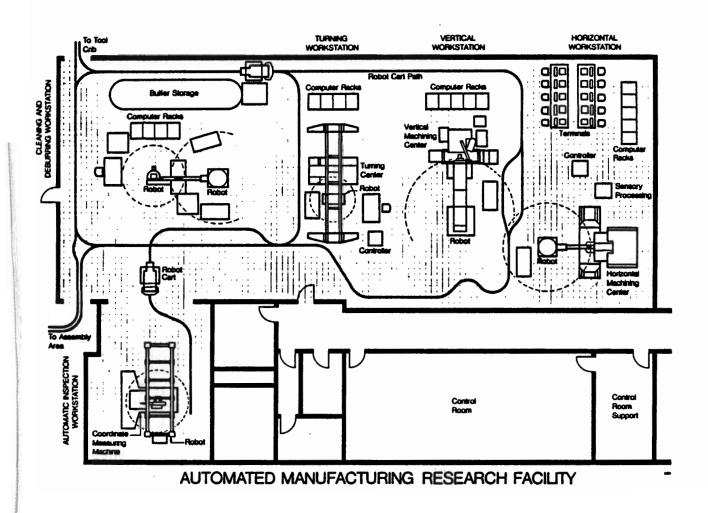
Figure 1. The Automated Manufacturing Research Facility.
