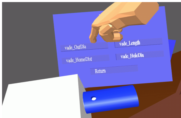
Figure 5. Parametric design modifications in VADE. The user selects the virtual menu button to modify the diameter of the indicated part.
