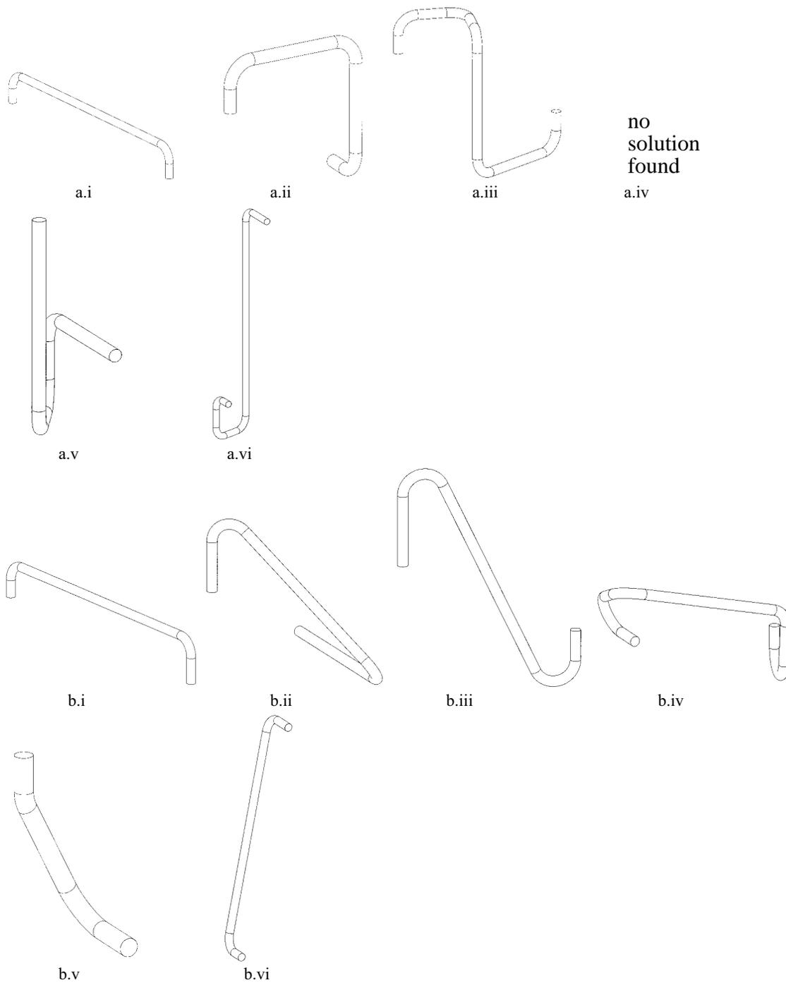
**Figure 2.** Tubes for layout of Figures 1: a) classification-based plane-orthogonal tubes and b) analogous simulated annealing-based tubes.
