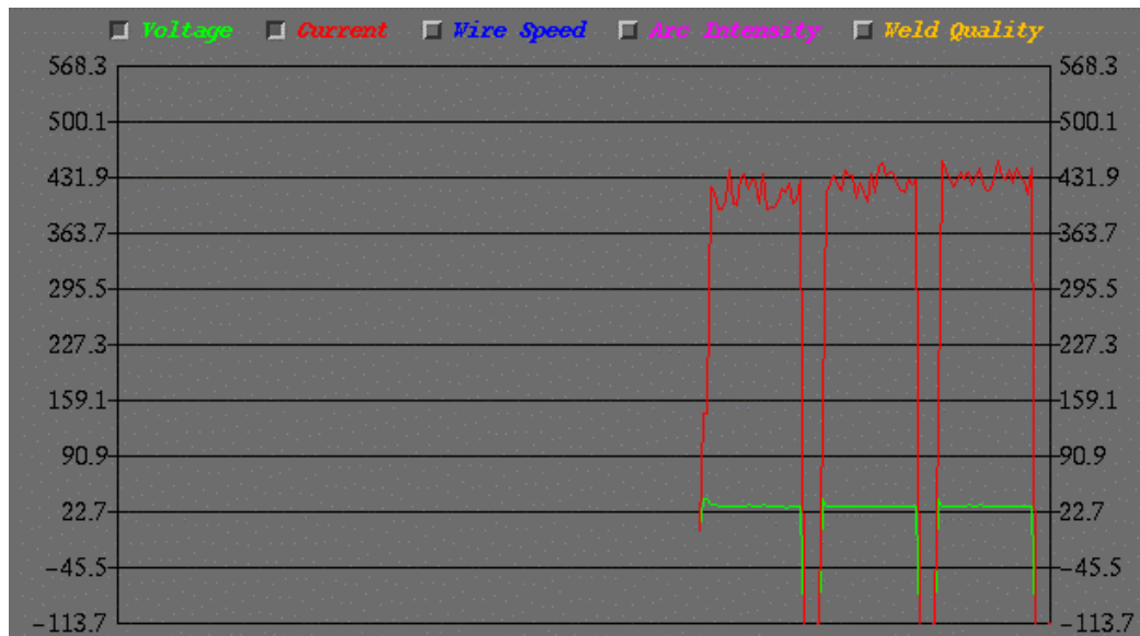
Figure 2: Weld current and voltage are plotted as the weld occurs. This is the same information available on the front panel of the power source.
