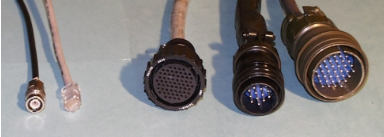
Figure 3. Multi-pin cables carrying analog signals can be replaced by network cables
