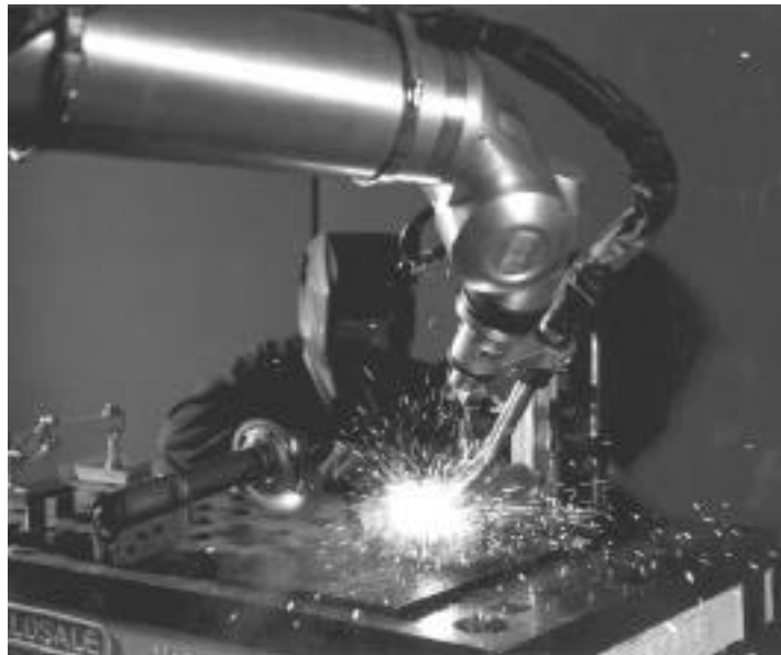
Figure 1: AWMS welding cell
