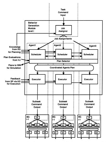
Fig. 3. Internal structure of a Behavior Generation (BG) module. A BG module is an organizational unit consisting of a Job Assignor, a set of Schedulers, a Plan Selector, a plan holding register that contains the coordinated agents plan, and a set of Executors. The Schedulers, Executors, and Job Assignors comprise agents within the BG units. Each agent is part of two BG units at two different levels. At level i, an agent is a team member, or peer. At level i-1, the same agent is a supervisor.
