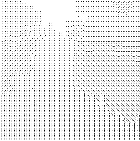
Figure 11: The optical flow plot for Figure 10. The flow on the floor shows clearly despite a lack of texture and sharp edges.
