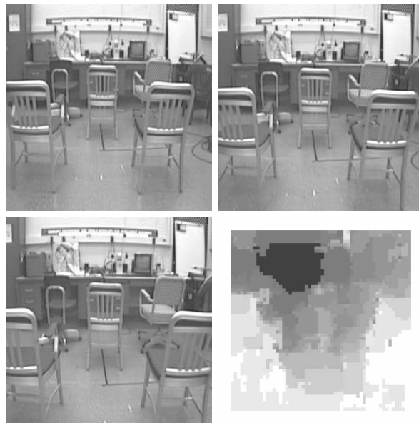
Figure 8: Three frames showing an approach to metal chairs, with a magnitude plot of the optical flow for the third frame; brighter points indicate faster motion.
