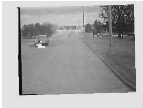
Figure 4: Stabilized frame with superimposed moving object regions.
