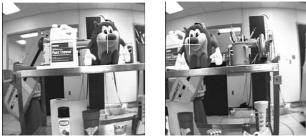
Figure 12: Example of locating a model object (stuffed doll) under conditions of motion, clutter, and perspective.
