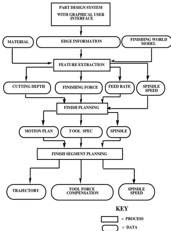
Figure 1. ADACS Finishing Process Model
