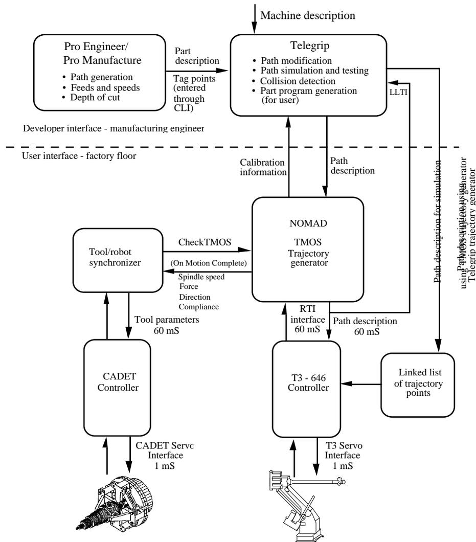
Figure 2. ADACS Control Structure
