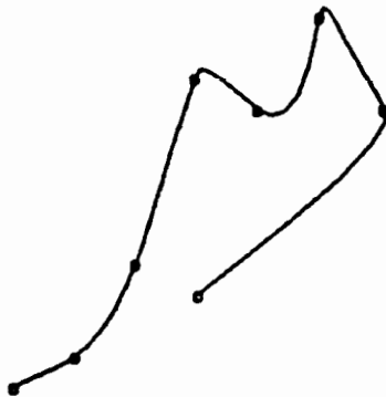
Figure 2 A curve generated using three points and a vector procedure. The vector defines the tangent value at the second point.
