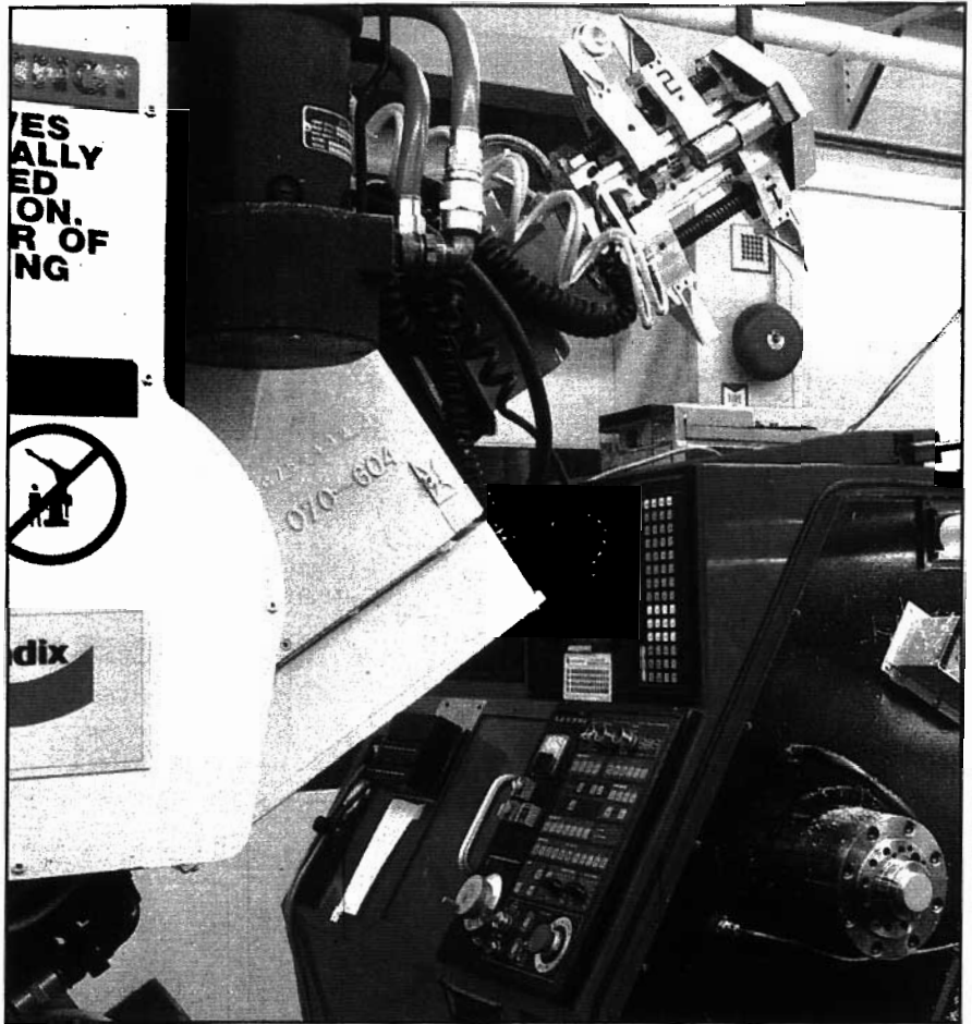
In the turning work station, an NBS-developed gripper is used to place part blanks and semi-finished parts in the collet of the turning center.
