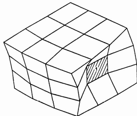
Fig. 5 Typical deformed shape of the workpart;  $N^f = 2$
