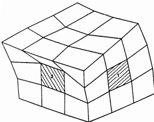
Fig. 2 Typical deformed shape of the workpart;  $N^f = 3$
