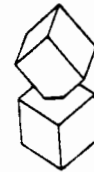
Figure 6. Even if no edge in the node from the master tree intersects a surface in the transformed tree, the nodes can intersect.
