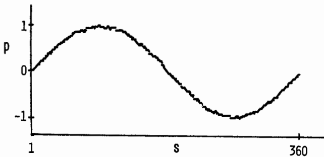
Fig. 6 After sixteen data points are stored. Maximum error = 0.09 and r.m.s. error = 0.033.
