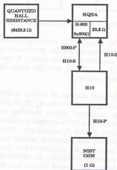
Fig. 1 Resistance Scaling from QHR to 1  $\Omega$ .
