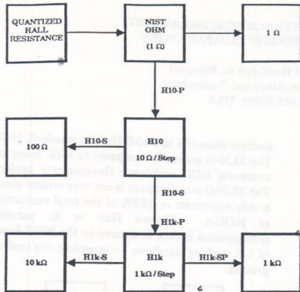
Fig. 2 Resistance Scaling to 1 kΩ and 10 kΩ.
