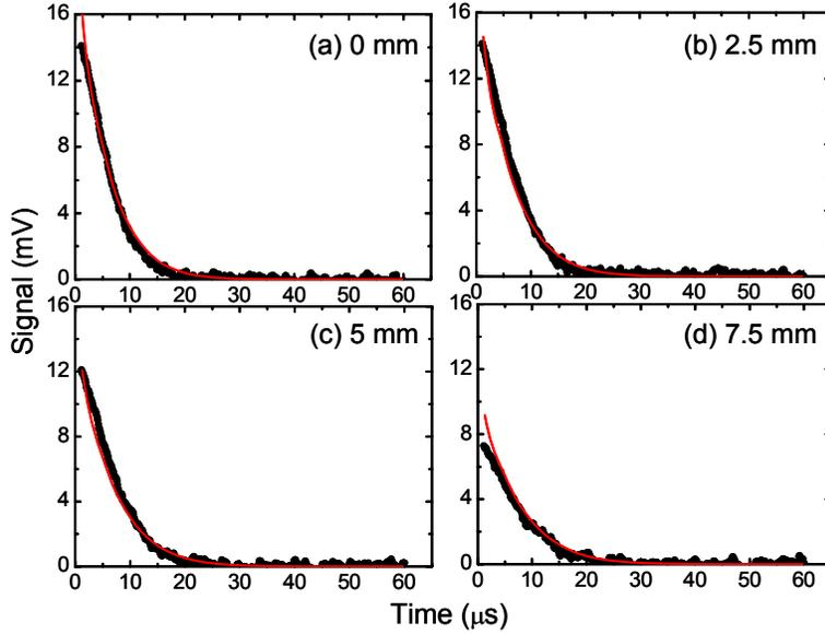
Fig. 5. 631 nm fluorescence decay at three detector positions relative to the laser-atom beam intersection. (a) 0 mm, (b) 2.5 mm, (c) 5 mm, and (d) 7.5 mm. Black dots indicate measurements, and red line indicates model used to extract lifetime. Extracted lifetime is  $5.6 \pm 1.4 \mu\text{s}$ .
