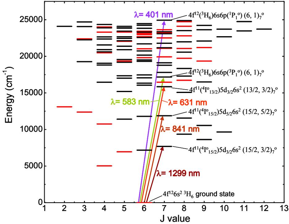
Fig. 1. Energy levels of erbium, showing five laser cooling transitions. Red horizontal lines indicate even parity states and black horizontal lines indicate odd parity states.
