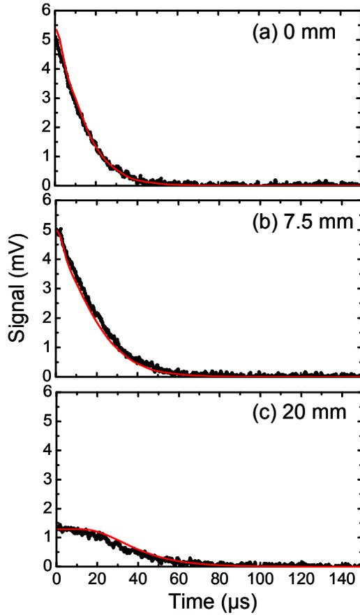
Fig. 4. 841 nm fluorescence decay at three detector positions relative to the laser-atom beam intersection. (a) 0 mm, (b) 7.5 mm, and (c) 20 mm. Black dots indicate measurements, and red line indicates model used to extract lifetime. Extracted lifetime is  $20 \pm 4 \mu\text{s}$ .
