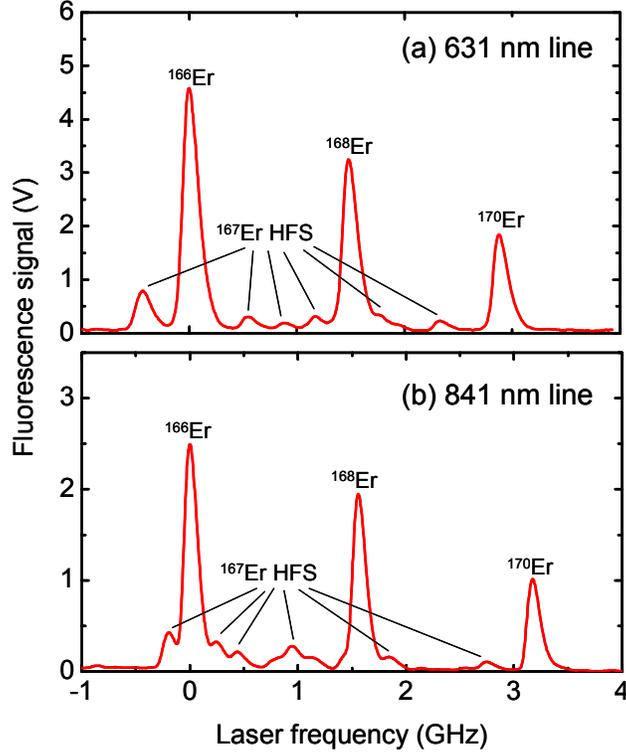
Fig. 3. Measured fluorescence spectra for (a) the 631 nm line and (b) the 841 nm line, showing the isotopes  $^{166}\text{Er}$ ,  $^{168}\text{Er}$  and  $^{170}\text{Er}$ , and the hyperfine structure (HFS) for  $^{167}\text{Er}$ .
