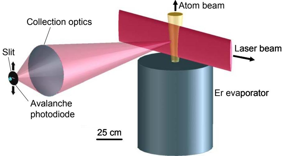
Fig. 2. Schematic of the crossed-beam experimental arrangement.
