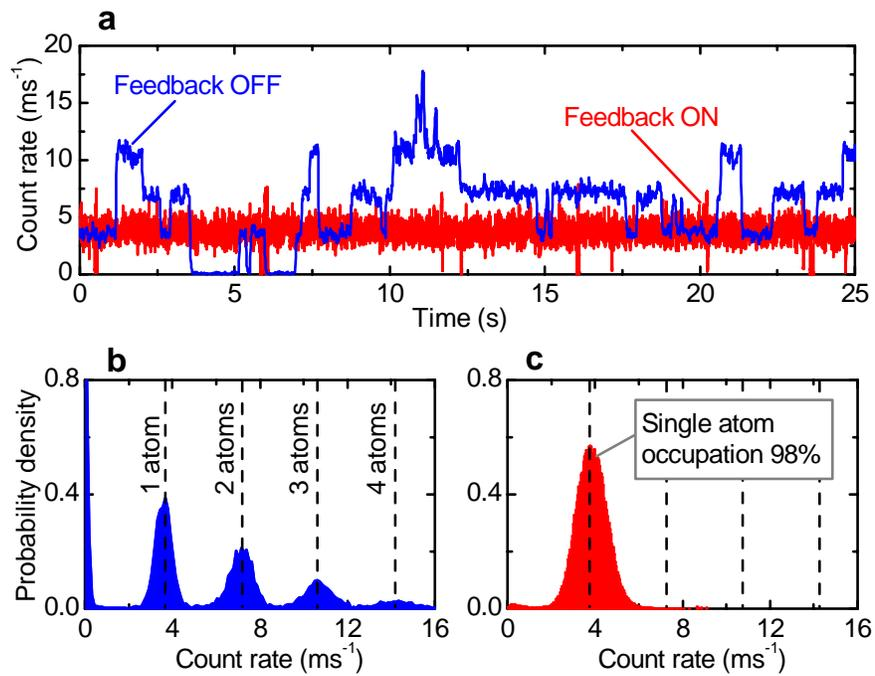
**Figure 1.** Fluorescence from a feedback-controlled single-atom magneto-optical trap. (a) Time series of feedback-off data showing random single atoms jumps, and feedback-on data showing constant, single-atom fluorescence. (b) Histogram of feedback-off data in 1(a). (c) Histogram of feedback-on data in 1(a). Note that the feedback-off data were collected with a much smaller load rate and longer detection time constant than feedback-on data.
