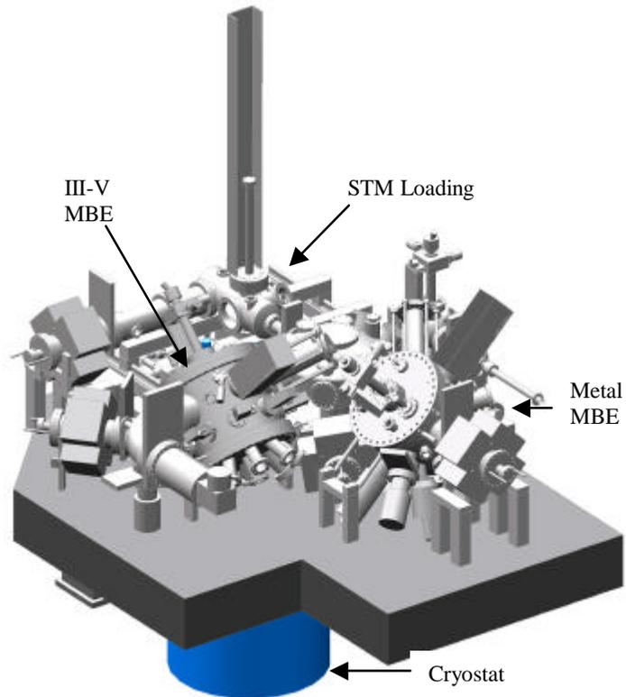
Fig. 1: CAD drawing of the NanoPhysics System.
