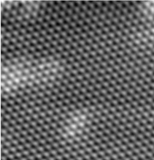
Fig. 3: Atomic resolution STM image, 6x6nm, of the Cu(111) surface obtained at 4.3 K. The grayscale range is 0.02 nm.
