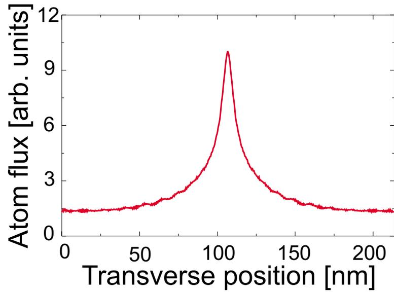
FIG. 1. Laser-focused chromium flux calculated within a semiclassical approximation by tracing trajectories of  $10^5$  atoms exiting an oven at 1900 K and collimated to a FWHM divergence of 0.16 mrad. The laser is detuned from the chromium two-level resonance by +500 MHz. A laser power of 20 mW is used, as this gives the best focusing, given the Gaussian laser  $1/e^2$  radius of  $60 \mu\text{m}$ .
