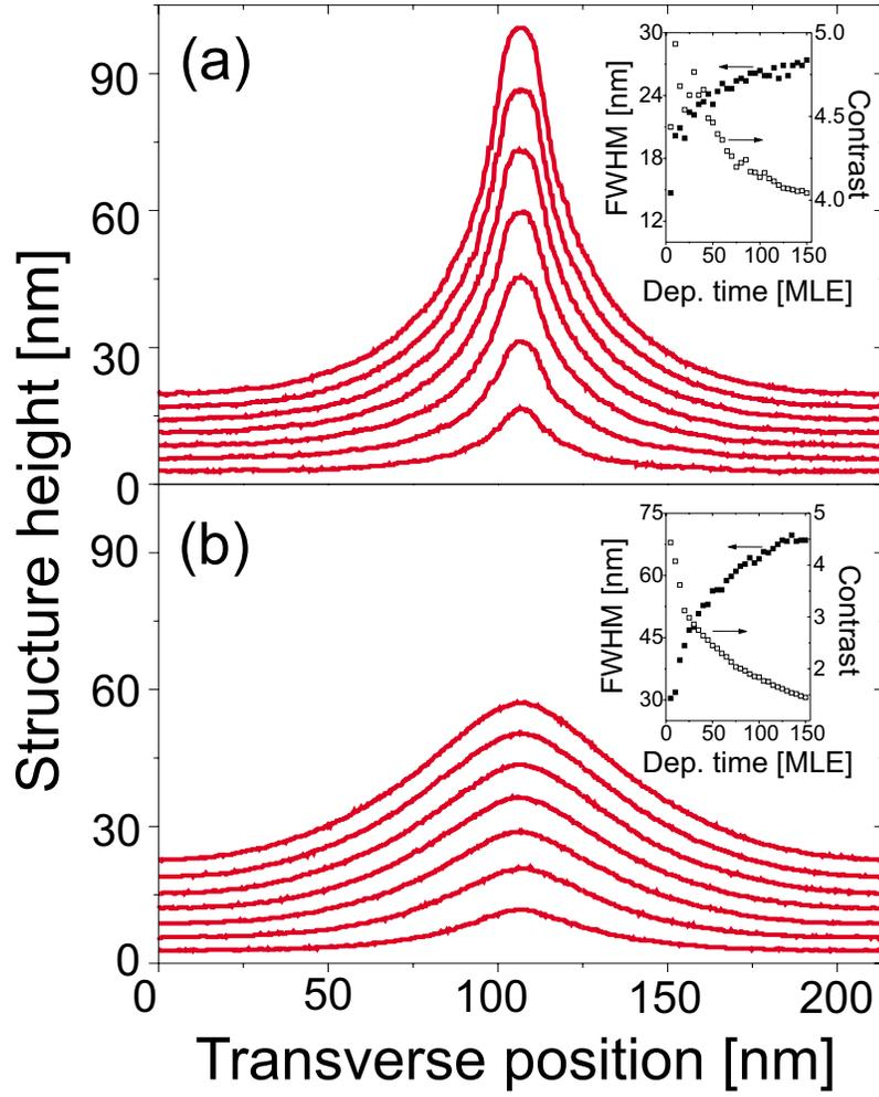
FIG. 2. Calculated TDS diffusion profiles for successive deposition times from 20 MLE to 140 MLE at 20 MLE intervals. (a) Substrate temperature  $T_S = 280$  K; (b) Substrate temperature  $T_S = 300$  K. The evolution of the structure FWHM and contrast with deposition times from 5 MLE to 150 MLE at 5 MLE intervals is shown in the insets.
