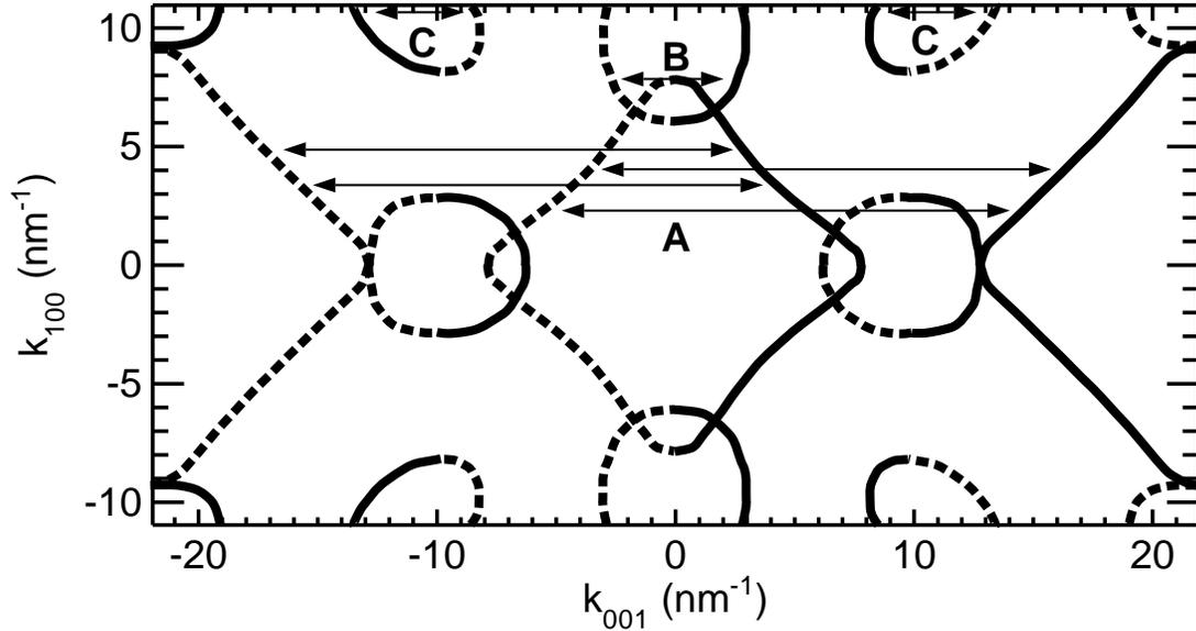
FIG. 1. Slice through Cr Fermi surface for an interface in (001) direction. The parts of the Fermi surface with states moving toward (away from) the interface are shown as solid (dashed) lines. Spanning vectors associated with several parts of the surface are shown as arrows and labeled.
