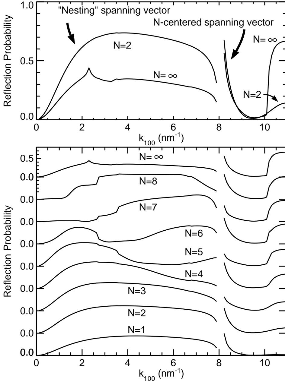
FIG. 4. State-to-state reflection probabilities for selected Cr electrons from Fe layers of finite thickness,  $N$  layers, embedded in bulk Cr. The bottom panel shows the reflection probabilities both for the states along  $\bar{\Delta}$  associated with the nesting of the Fermi surface and for the states at the  $N$ -centered ellipsoids. The top panel shows the same results for just a two layer thick Fe film and bulk Fe.
