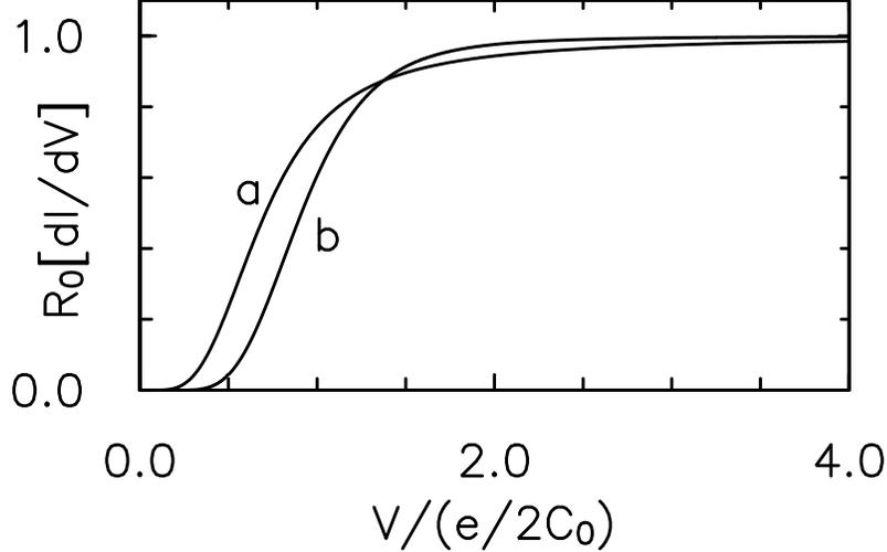
FIG. 4. Comparison of the differential conductivity for (b) an ideal transmission line with  $g = 10$  and (a) a resistive transmission line with  $r = 8000 \text{ } \Omega/\mu\text{m}$ ,  $\ell = 600 \text{ fH}/\mu\text{m}$ , and  $c = 0.022 \text{ fF}/\mu\text{m}$ .
