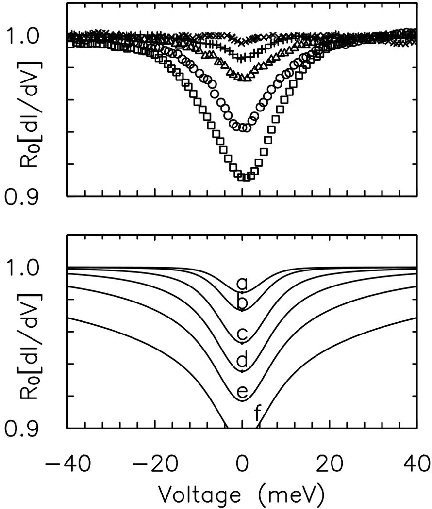
FIG. 8. Comparison of theory and the measurements of Gregory [22]. The bottom panel shows the calculated conductivity of isolated junctions with a series of different charging energies ( $E_C =$  (a) 0.1, (b) 0.2, (c) 0.5, (d) 1.0, (e) 2.0, (f) 5.0 meV) plotted as a function of voltage. The details of the calculation are discussed in the text. The top panel shows the measured conductivity for five different junctions.
