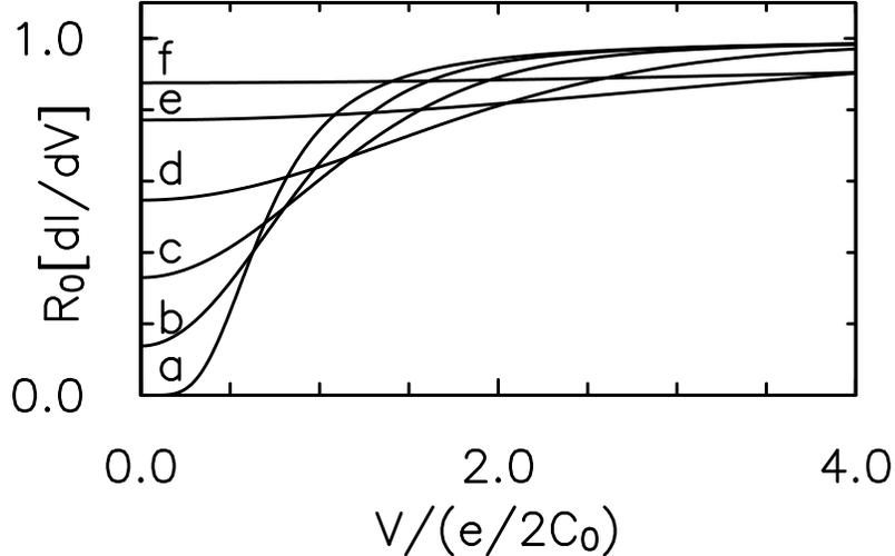
FIG. 5. Temperature dependence of the differential conductance for a resistive transmission line as in Fig. 4. The temperatures are (a) 0K, (b) 0.5K, (c) 1.0K, (d) 2.0K, (e) 5.0K, (f) 10.0K. The charging energy of the junction is 0.4 meV or  $4.6 \text{ K} \cdot k_B$ .
