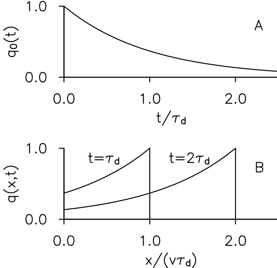
FIG. 2. Classical time dependence of a charge suddenly placed on a junction connected to an ideal transmission line. Panel A shows the decay in time of the charge remaining on the junction and Panel B shows the classical charge wave propagating down the transmission line. The quantity  $v = 1/\sqrt{\ell c}$  is the speed of light in the transmission line.
