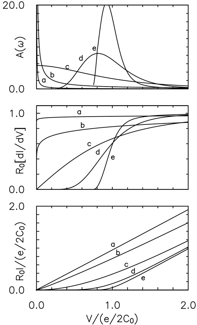
FIG. 3. Ideal transmission lines. The excitation spectrum  $A(\omega)$ , the differential conductivity  $dI/dV$ , and the current  $I$  are plotted for a series of transmission lines with coupling constants,  $g = 2Z/R_H$ , (a)  $g = 0.01$ , (b)  $g = 0.1$ , (c)  $g = 1.0$ , (d)  $g = 10$ , and (e)  $g = 100$ . The curves are scaled by the differential resistance of the junction in absence of charging effects,  $R_0$ , and by the voltage characteristic of the charging energy  $e/2C_0$ .
