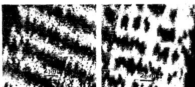
FIG. 2. SEMPA images of (a) \text{Co}_{86}\text{Cr}_{12}\text{Ta}_2 and (b) \text{Co}_{75}\text{Ni}_{25} films. The images are of the magnetization component along the track.
