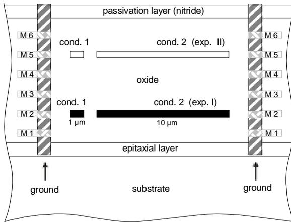
Fig. 1. Cross section of the asymmetric coupled lines.
