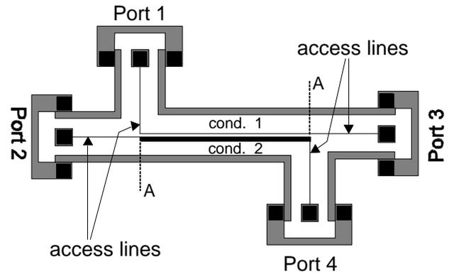
Fig. 2. Top view of the test structures.
