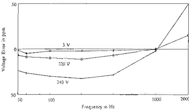
Fig. 5. Frequency response of voltage module
