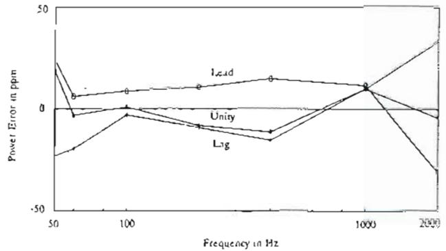
Fig. 6. Frequency response of power measurements.
