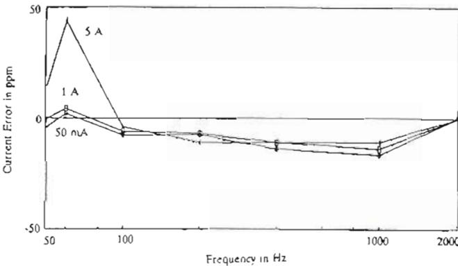
Fig. 4. Frequency response of current module.
