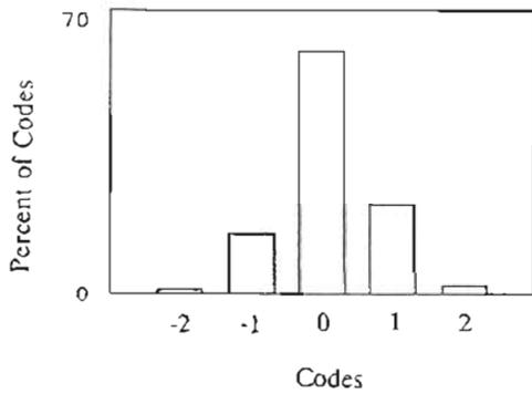
Fig. 3. Typical distribution of voltage codes for shorted input.
