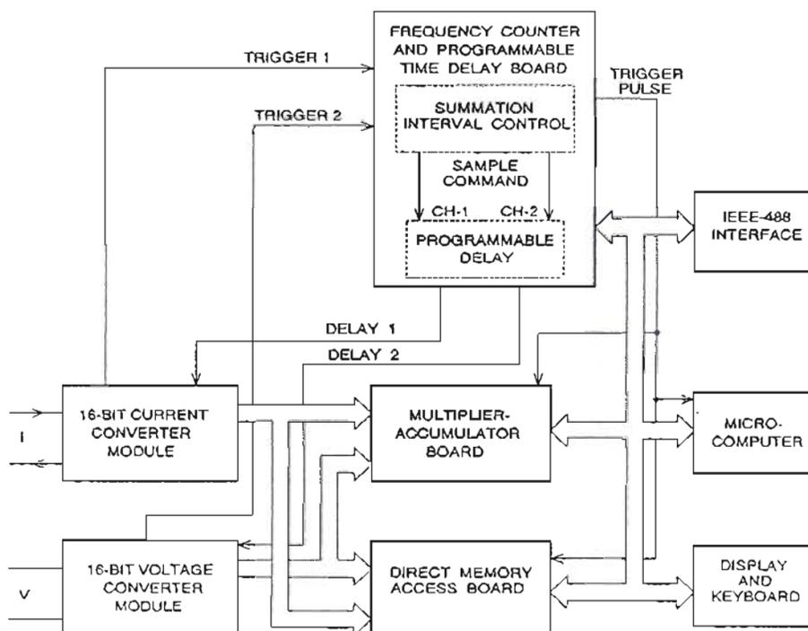
Fig. 1 Block diagram of the NIST high-accuracy sampling wattmeter
