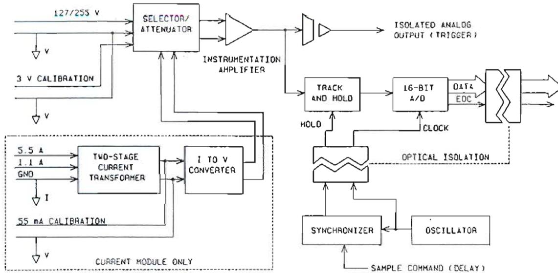
Fig. 2. Block diagram of the voltage and current input modules.
