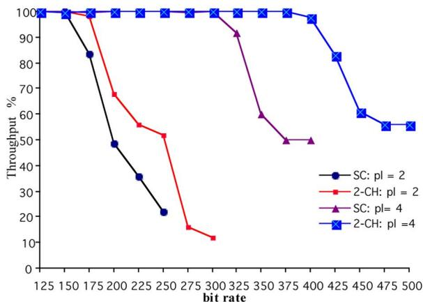
**Fig. 3.** Performance comparisons between SC and switching 2-CH switching system for path-loss (pl) factor of 2 and 4.
