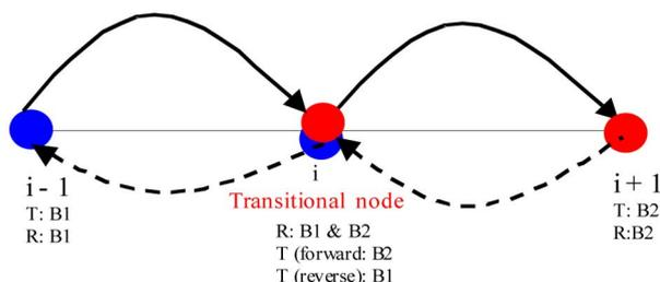
**Fig. 4.** Partitioning of a multihop link via the proposed transitional node.
