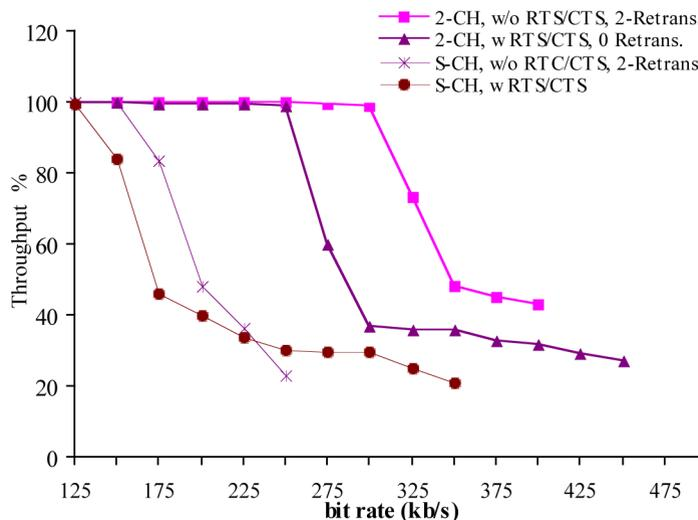
Fig. 11. RTS/CTS effects on single-channel and 2-CH partitioning [configuration (a) with  $pl = 2$ ].
