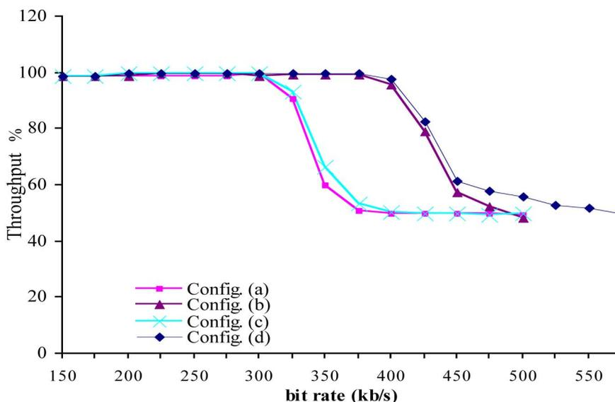
**Fig. 7.** Throughput performance of the two-channel systems corresponding to configurations (a)–(d) in Fig. 3 for propagation factor of  $pl = 4$ .
