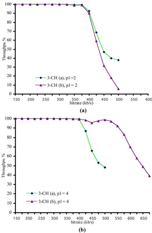
Fig. 9. Throughput performance of the 3-CH system corresponding to configurations (a) and (b). (a)  $pl = 2$  and (b)  $pl = 4$ .
