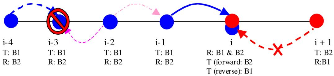
Fig. 10. Hidden node effect in link partitioning.
