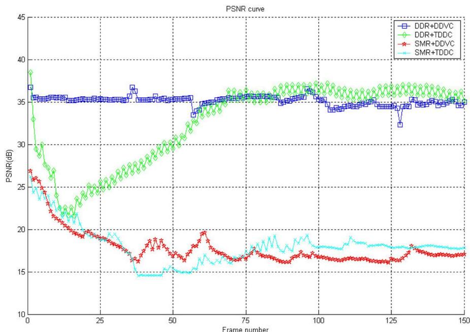
Fig. 20. Objective quality comparison of different encoders using different routing protocols: “Coastguard.”
