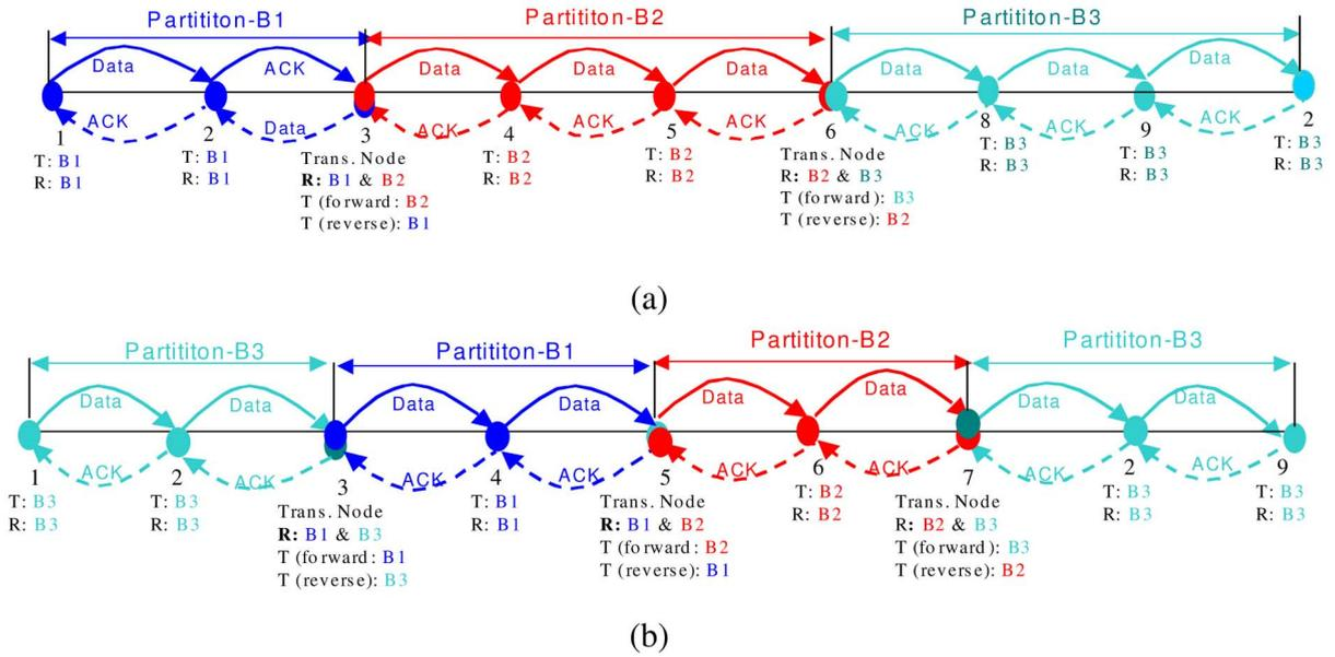
Fig. 8. Three-channel partitioning systems: (a) two-hop and (b) three-hop configuration.
