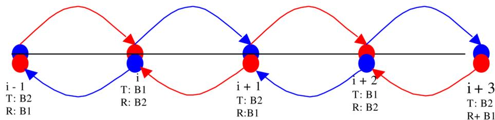
Fig. 2. Single NIC, half duplex, two channel switching system with systematic channel assignment for transmission and reception of data and acknowledgment (ACK) packets.
