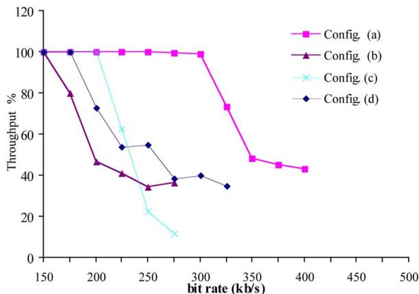
**Fig. 6.** Throughput performance of the two-channel systems corresponding to configurations (a)–(c) in Fig. 3 for path-loss factor of  $pl = 2$ .
