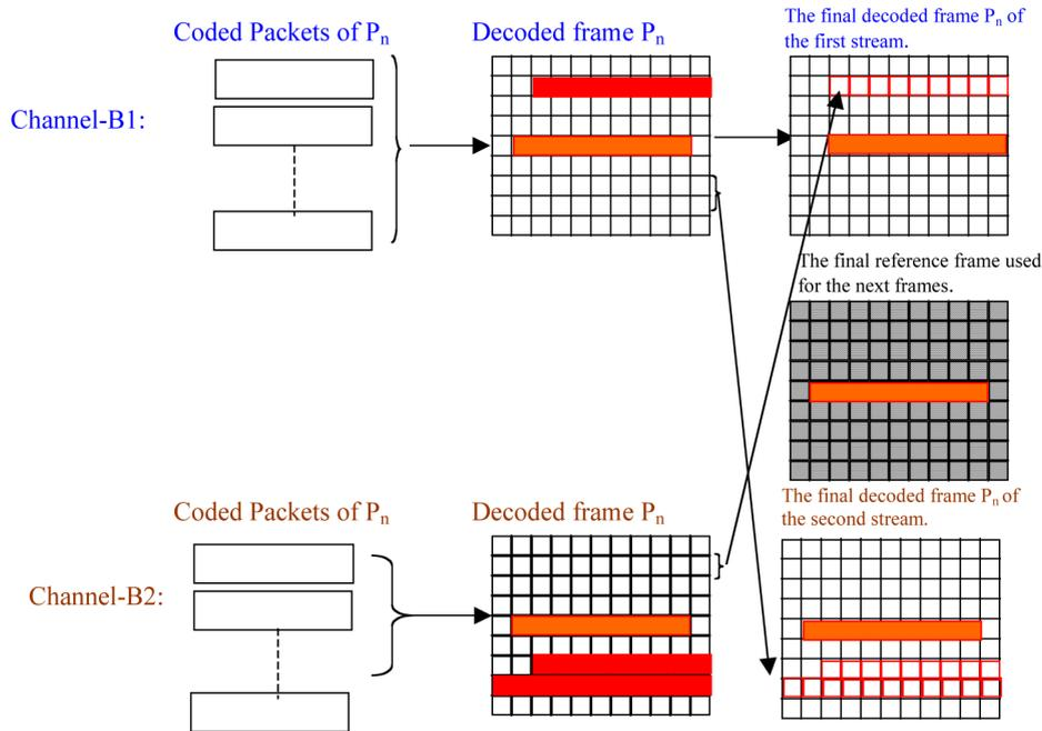
Fig. 15. Bitstream combiner for packet-loss recovery in duplicate decoder.
