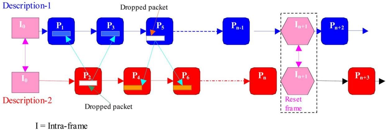
**Fig. 14.** Temporal-based dual description coding with packet concealment arrangements.
