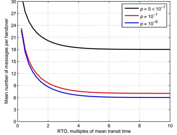
Fig. 8. Mean number of messages generated by MIH signaling endpoints using TCP transport during a handover where  $M = 3$  and  $K = 6$ , for various RTO values.
