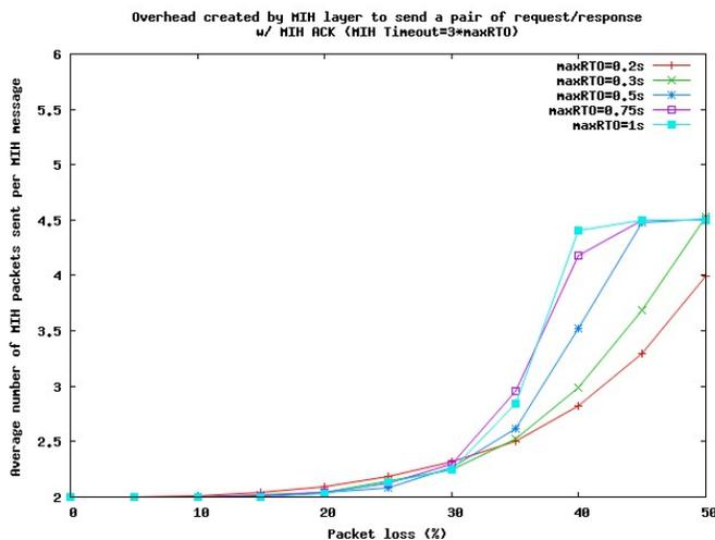
Fig. 21. Simulation values of MIH overhead for Request/Response exchanges over TCP with MIH ACKs.
