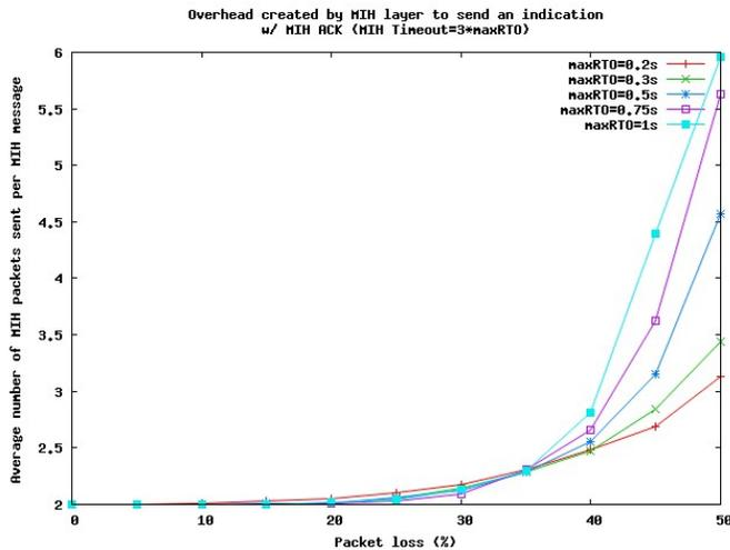
Fig. 20. Simulation values of MIH overhead for Indication messages over TCP with MIH ACKs.
