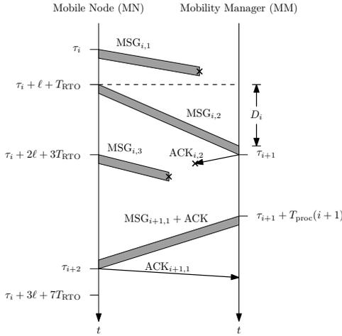
Fig. 5. Sample MIH signal flow between MN and MM when TCP transport is used and when some messages and TCP ACKs are lost in transit.
