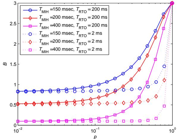
Fig. 11. Plot of  $\bar{B}$ , the average size of the message backlog generated by MIH retransmissions due to expiration of the MIH timer, versus  $p$ , the probability of message loss for different values of the MIH timeout,  $T_{MIH}$ .
