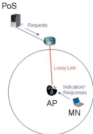
Fig. 12. Network topology used in simulations of Indication and Request/Response MIH message exchanges.
