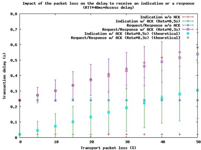
Fig. 14. Theoretical and simulation values of mean MIH handover time for MIH handovers where  $M = 1$  (Indication) and  $M = 2$  (Request/Response) over UDP.
