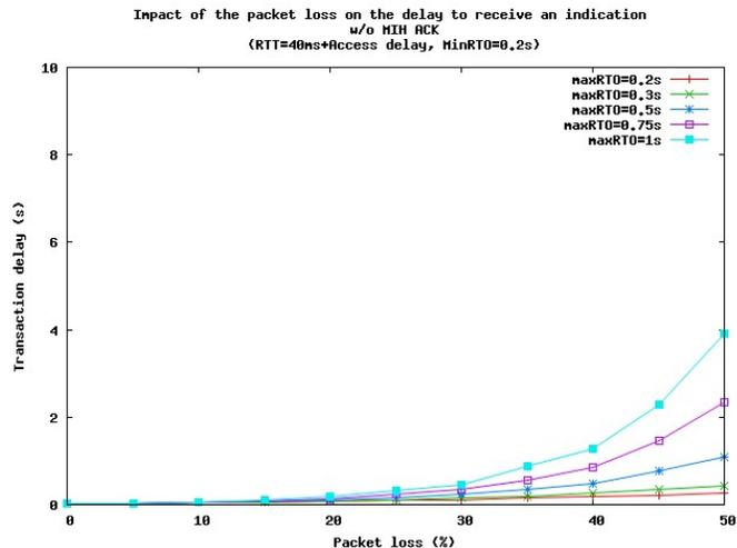
Fig. 17. Mean MIH Indication transaction completion time over TCP transport without MIH timeouts and acknowledgments.
