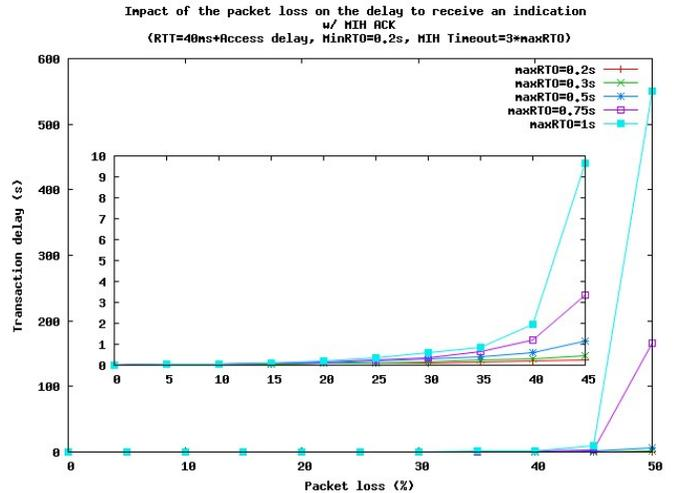
Fig. 15. Mean MIH Indication transaction completion time over TCP transport with MIH timeouts and acknowledgments.
