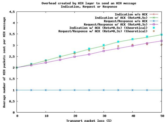
Fig. 19. Theoretical and simulation values of MIH overhead for Indication and Request/Response exchanges over UDP.
