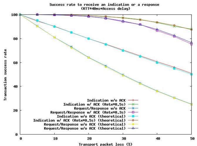
Fig. 13. Theoretical and simulated values for MIH transaction completion probability.
