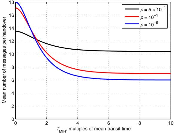
Fig. 4. Mean number of messages generated by MIH signaling endpoints during an exchange where  $M = 3$  and  $R_i = 2$  for  $i = 1, 2, 3$ .
