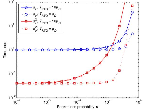
Fig. 7. Mean and variance of the handover time  $H$  versus packet loss probability,  $p$ , for short and long TCP RTO values ( $T_{\text{RTO}} = \mu_D$  and  $T_{\text{RTO}} = 10\mu_D$ , respectively).
