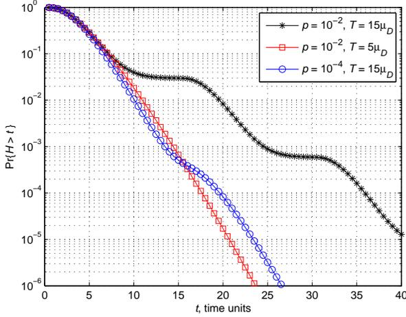
Fig. 2. Probability that the handover time,  $H$ , exceeds  $t$  seconds for three sets of values of packet loss probability  $p$  and MIH timeout,  $T$ .
