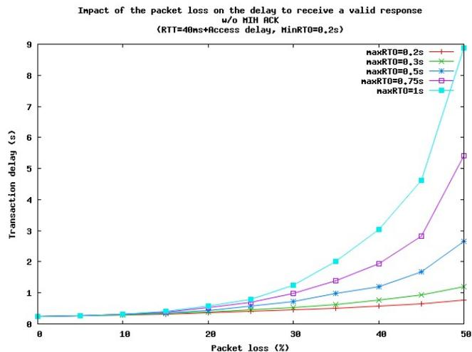
Fig. 18. Mean MIH Request/Response transaction completion time over TCP transport without MIH timeouts and acknowledgments.
