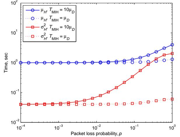
Fig. 3. Mean and variance of the handover time  $H$  versus packet loss probability,  $p$ , for short and long MIH timeout values ( $T_{\text{MIH}} = \mu_D$  and  $T_{\text{MIH}} = 10\mu_D$ , respectively).
