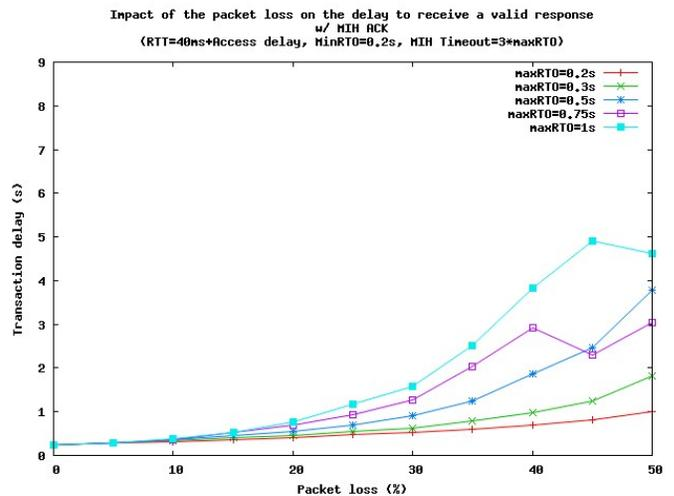
Fig. 16. Mean MIH Request/Response transaction completion time over TCP transport with MIH timeouts and acknowledgments.
