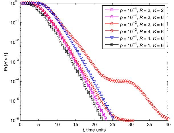
Fig. 6. Probability that the MIH message exchange time,  $H$ , exceeds  $t$  seconds for six sets of values of packet loss probability  $p$ , RTO, and number of RTO stages,  $K$ .
