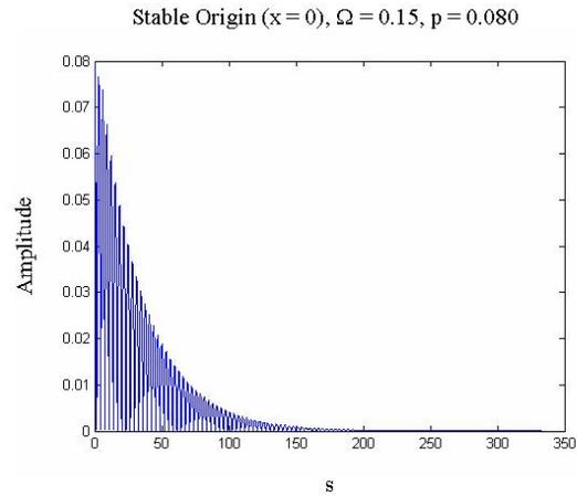
**Fig. 12.** Stable Amplitude of Solution at Point M
