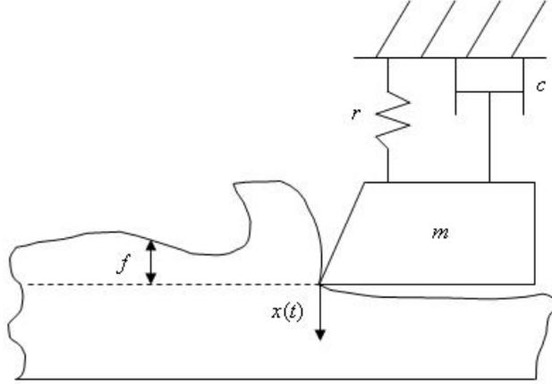
Fig. 3. One Degree-of-Freedom-Model for Single-Point Turning
