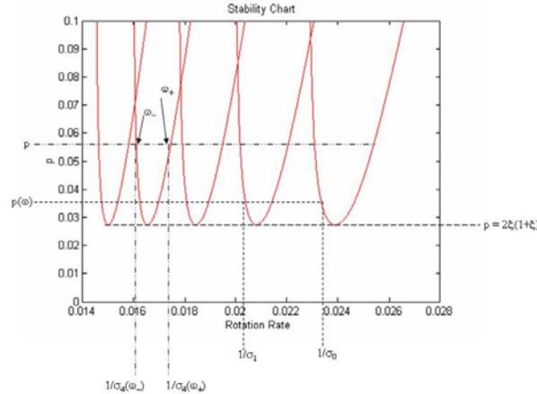
Fig. 4. Stability Chart with Sample Critical Eigen Triples Identified
