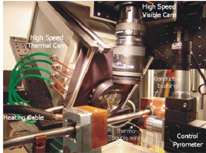
Figure 4. Central region of NIST SHPB, showing instrumentation used to heat sample and to control and measure sample temperature.
