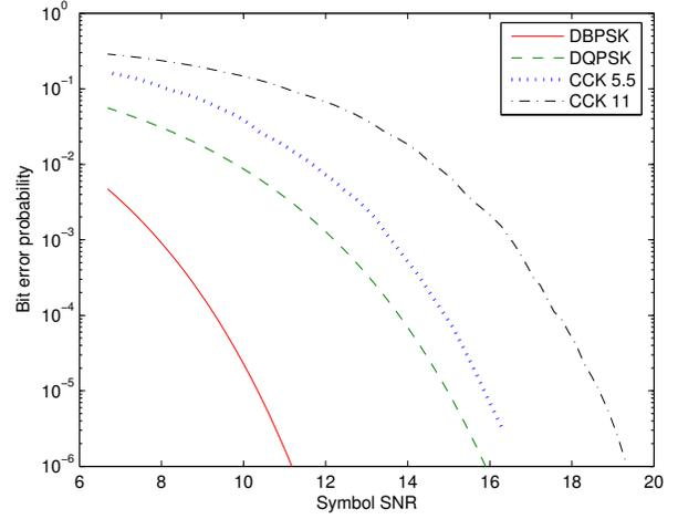
Fig. 2. Bit error rate vs. SNR of 802.11b data rate modes in AWGN
