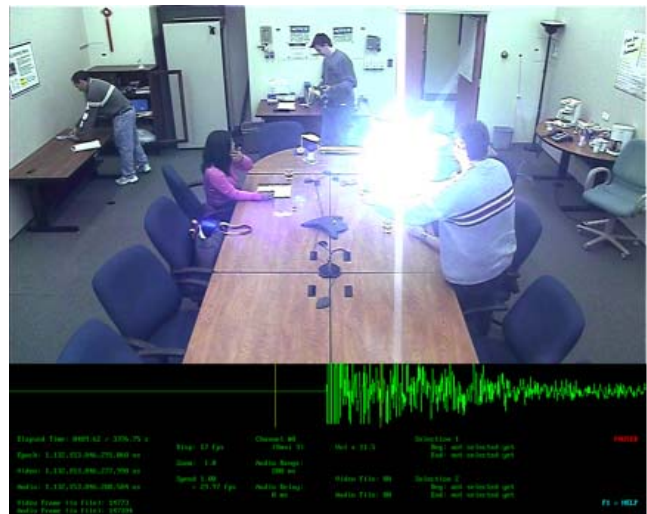
Figure 5: Resynchronization tool showing the video flash and audio clap from indices after resynchronization process. The Synchronization tool allows the operator to determine delay between audio and video by allowing the audio delay to be varied until the clap impulse is visible in the flash frame
