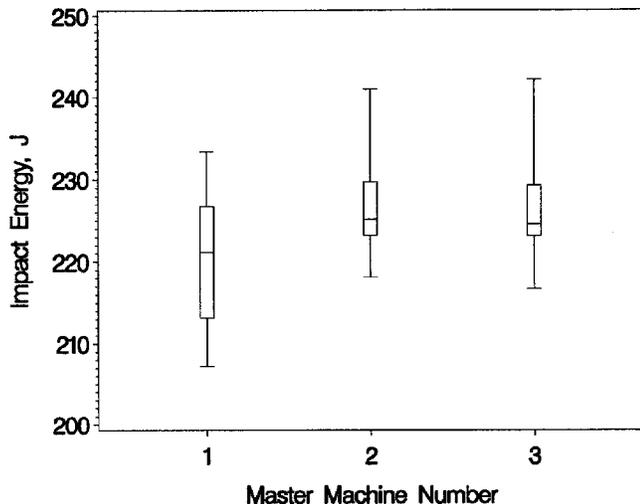
FIG. 1—Distribution of verification set measurements for each master machine.
