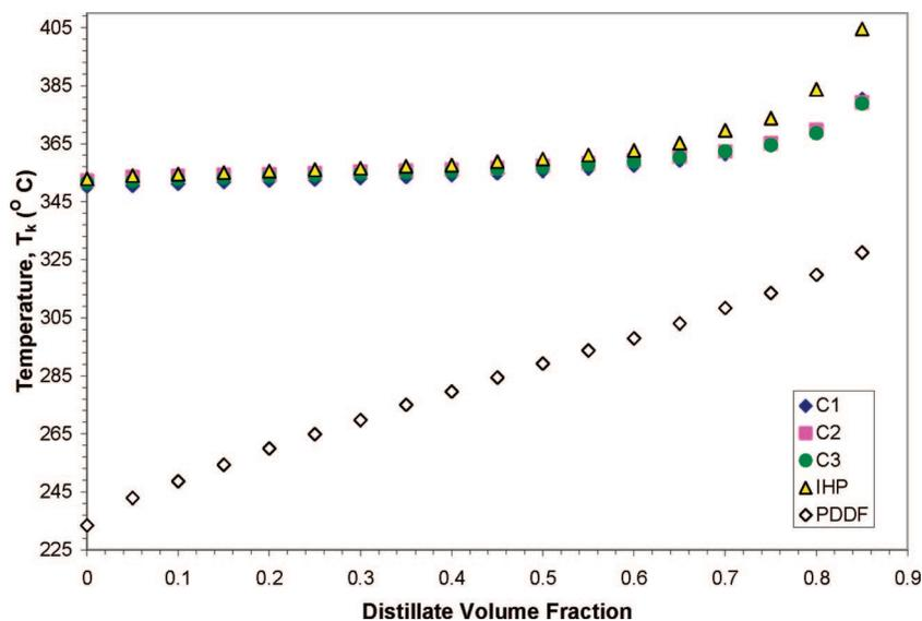
**Figure 4.** Distillation curves of the four biodiesel fuel samples and the petroleum-derived diesel fuel (PDDF) sample. The uncertainty on the temperature measurements is smaller than the symbols used.
