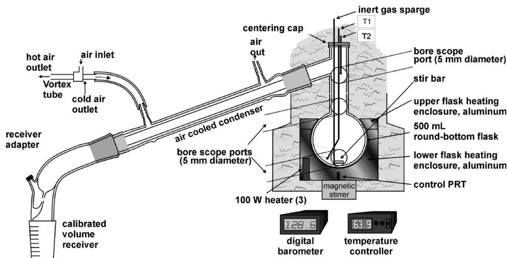
Figure 1. Distillation curve apparatus with inert gas sparge.
