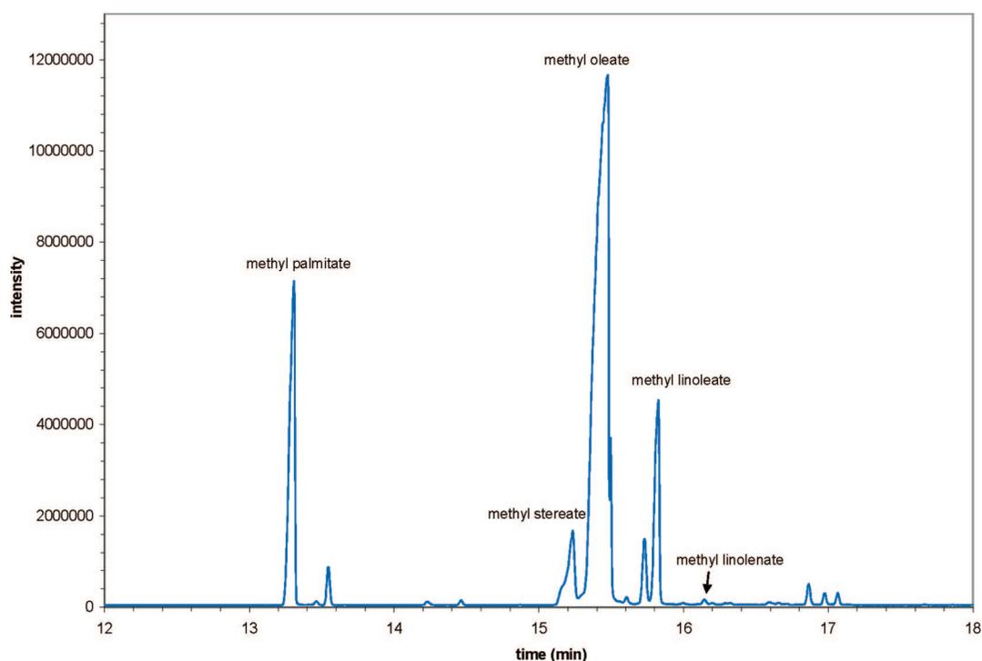
**Figure 3.** Uncalibrated total ion chromatogram of the 50% distillate volume fraction for the IHP biodiesel fuel. The five main FAMES present in biodiesel are labeled; the predominant peak at 15.4 min is methyl oleate.
