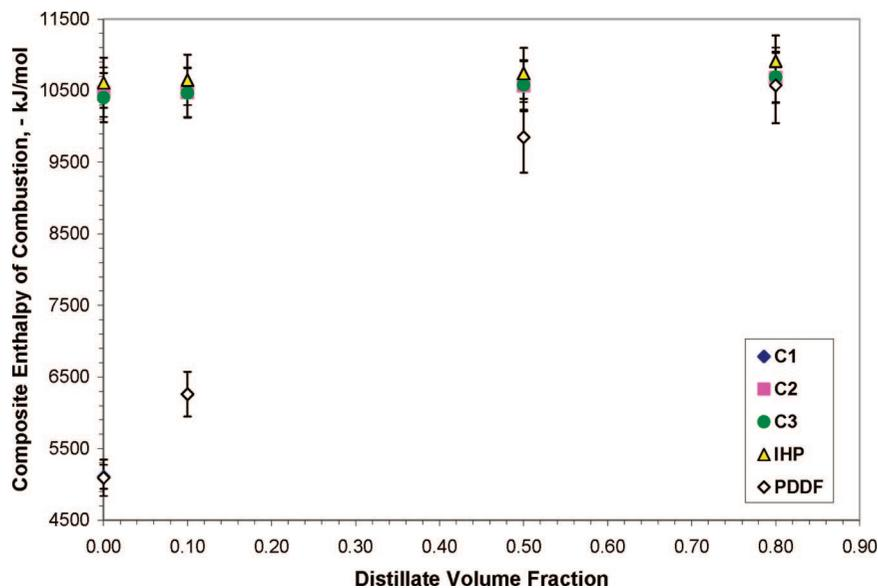
**Figure 5.** Enthalpy of combustion ( $-kJ/mol$ ) of the petroleum-derived diesel fuel and four biodiesel fuel samples. For the first drop of the petroleum-derived diesel fuel and C1 biodiesel fuel, the symbols overlap.
