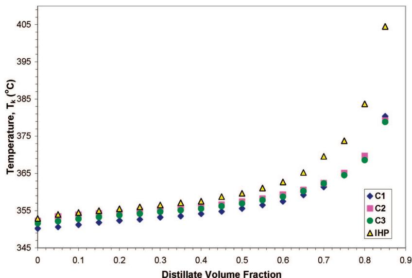
**Figure 2.** Distillation curves for each of the four biodiesel fuel samples. Each single curve shown for a given sample is representative of data collected for 3–6 distillation curves. The error bars on the temperature measurement are smaller than the symbols used.
