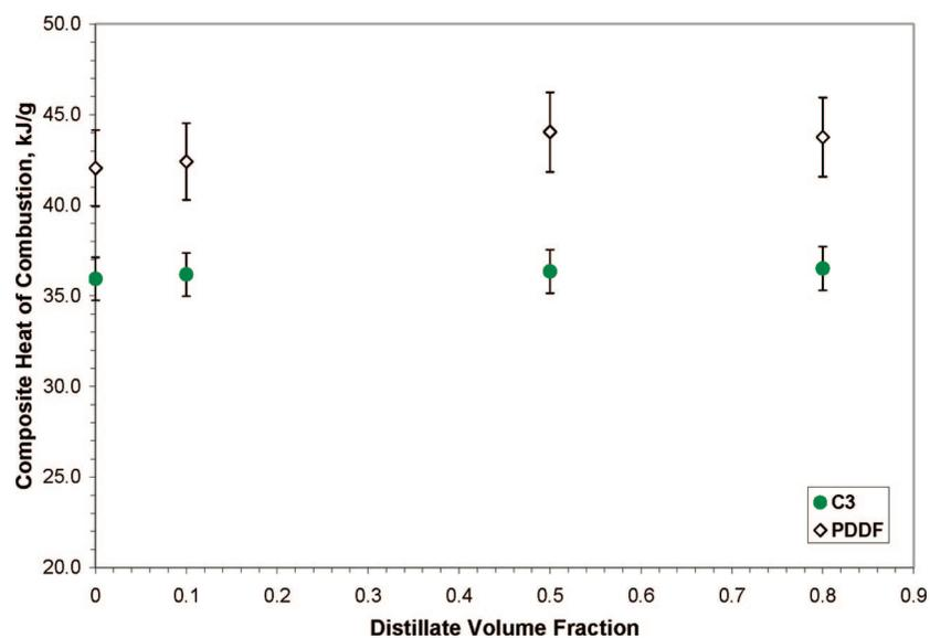
**Figure 6.** Enthalpies of combustion ( $-kJ/g$ ) of one representative biodiesel fuel sample (C3) and the distillate fractions of the petroleum-derived diesel fuel (PDDF).
