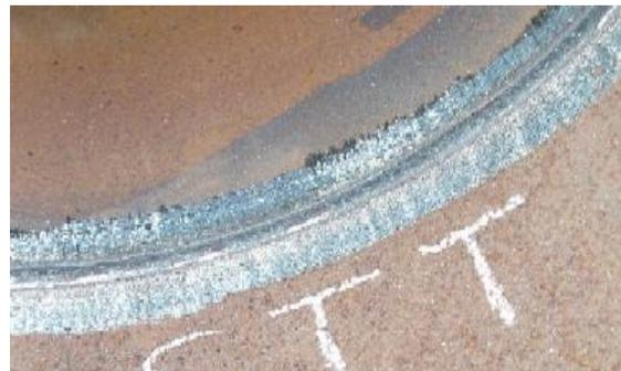
Figure 6 The face of the STT root weld (note the smooth appearance of the weld surface, without any cracks)
