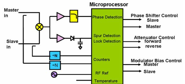
Figure 11. Proposed automatic control of the DIFO.
