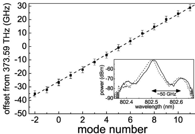
Fig. 4. Mode frequency versus mode number (solid squares) and expected dependence for the 5.000994 GHz repetition rate (dashed line). Error bars represent the frequency repeatability of the OSA. Inset: spectra of modes number 1 (solid curve) and 2 (dashed curve).
