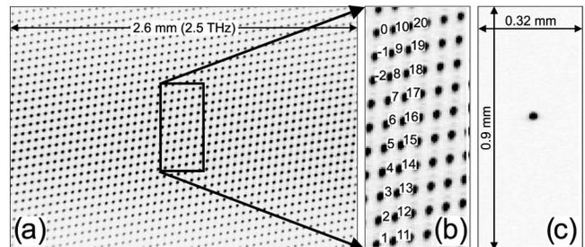
Fig. 3. (a) Output of the VIPA spectrometer recorded with a CCD camera. The image covers  $\sim 5$  nm centered at  $\sim 802.5$  nm. (b) Zoom into the CCD image. Successive modes are numbered. (c) Mode 1 isolated with a pinhole.
