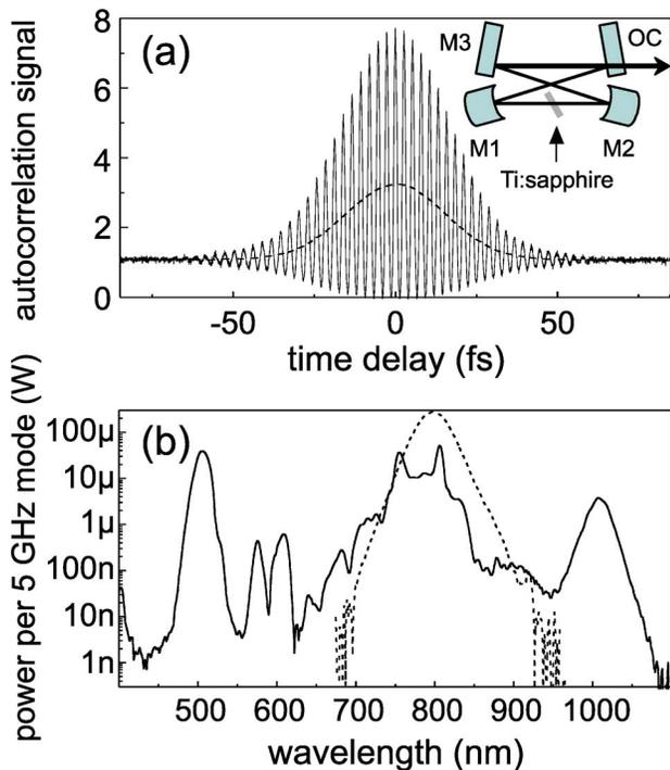
Fig. 1. (Color online) (a) Interferometric autocorrelation trace (solid curve) of the 5 GHz pulses and low-pass filtered trace (dashed curve). Inset: laser cavity schematic. (b) Laser output spectrum in units of power per 5 GHz mode (dashed curved) and octave-spanning spectrum after nonlinear broadening (solid curve).
