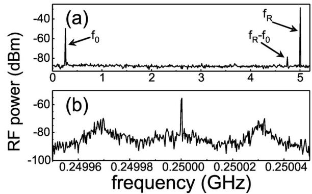
Fig. 2. (a) Self-referencing beat signal of the 5 GHz laser. Resolution bandwidth (RBW) is 300 kHz. (b) Phase-locked  $f_0$  signal with RBW set to 100 Hz.
