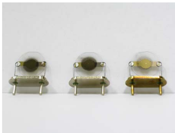
Figure 1. QCM devices coated with carbon nanotubes ( i.e. , black coating covering the gold electrode in the center of each crystal). From left to right: the crystals have been heated to temperatures of 375 °C, 400 °C, and 425 °C, with significant mass loss occurring at 425 °C. In this latter case, the underlying gold electrode is clearly visible.
