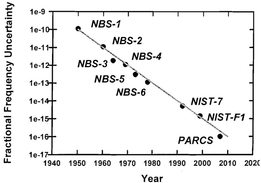
Fig. 1. The inaccuracy of typical primary frequency standards based on the cesium atom hyperfine transition. The slope of the line represents an improvement of about a factor of 10 in accuracy per decade
