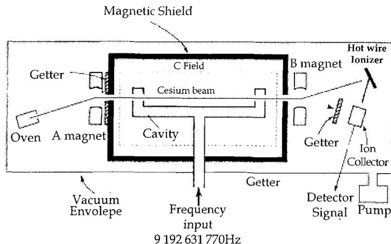
Fig.2. Diagram of a cesium-beam frequency standard using magnetic state-selection and detection. The form of Ramsey interrogation involves a U-shaped microwave cavity (the Ramsey cavity) where the microwave interrogation fields are spatially separated
